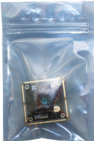
Place Camera Sample into Anti-Static Bag
